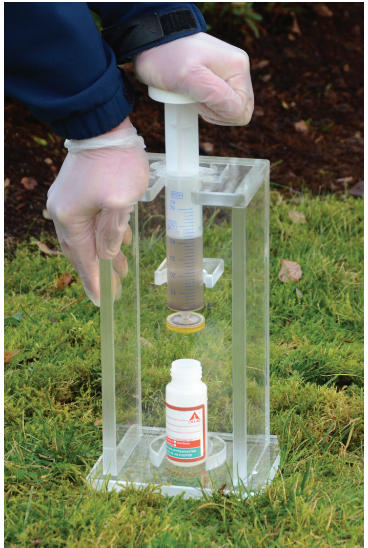
Field filtration of dissolved metals by syringe filter
