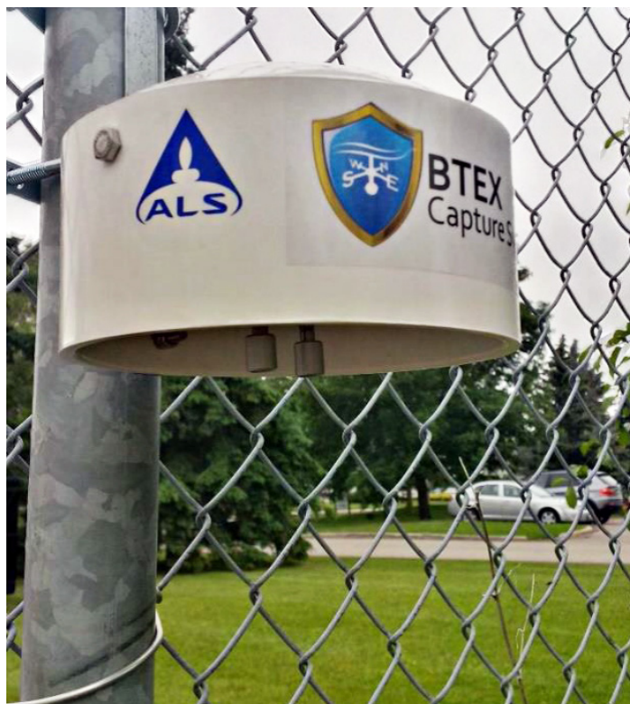
Fig. 1. Passive TD tubes in a shelter
